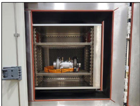
Figure 3: NovA Platform in thermal shock cabinet.
