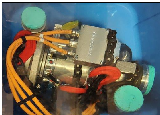
Figure 6: NovA Platform during ingress protection (IP) test.
