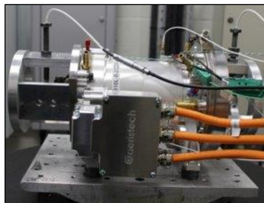
Figure 5: NovA platform on shaker test rig.
