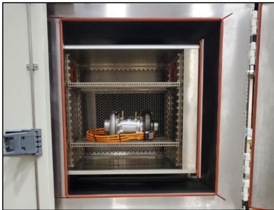
Figure 3: NovA Platform in thermal shock cabinet.
