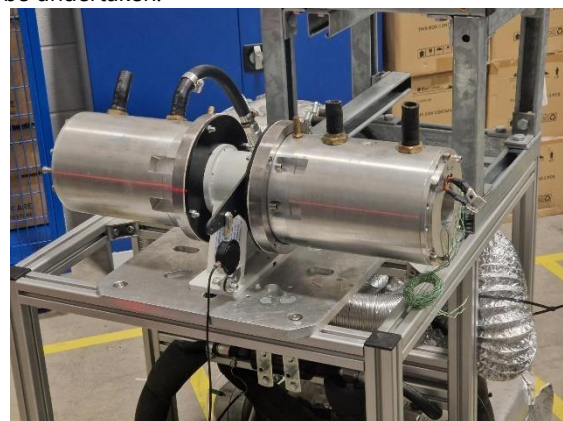
Figure 1: Sub-system testing of e-magnetics. Nose-to-nose motor arrangement with torque arm and load cell.
