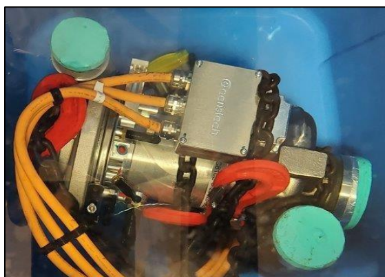
Figure 6: NovA Platform during ingress protection (IP) test.
